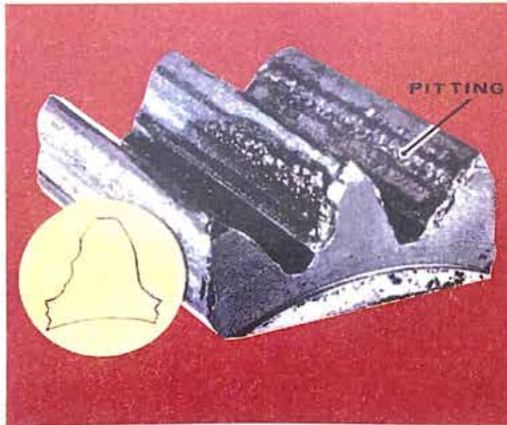
Figure 28. Advanced stage of abrasive wear.
