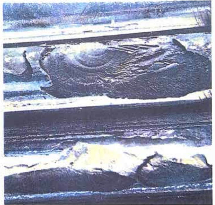
Figure 11. Midtooth fracture caused by pitting.
