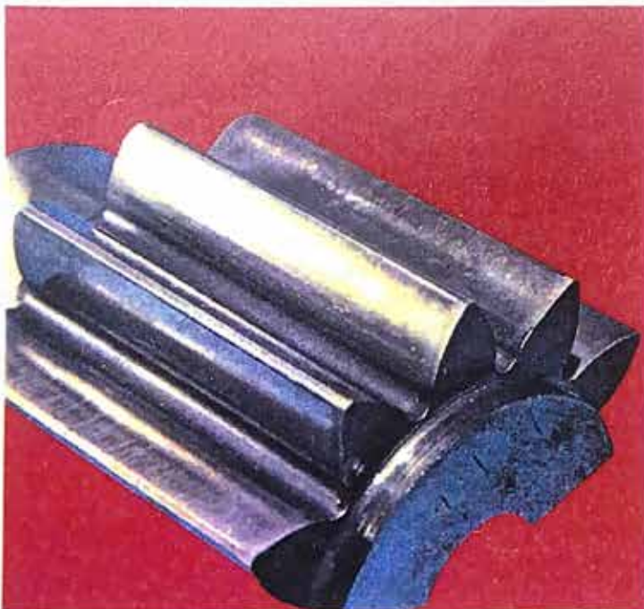
Figure 18. Pitting and wear.
